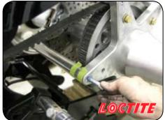
10. Install lower swing arm mounting bolts both side leave loose. Install upper swing arm mounting bolts, make sure to put the washer between the swing arm and the star plate on both sides leave loose. Refer to diagram for placement of washers and spacers.
