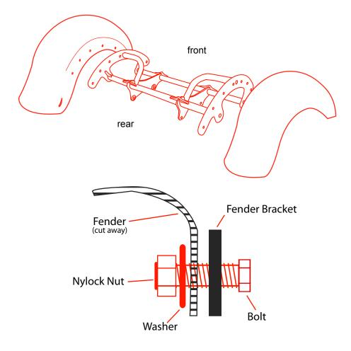
18.Remove two bolts and lock nuts just below bolts previously removed, on one side at a time. Install fender and bracket on the rear end.
