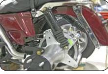
13. Install brake line to rear caliper and bled.
