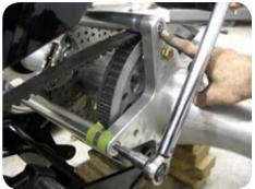
11. Install lower swing arm mounting bolts both side leave loose. Install upper swing arm mounting bolts, make sure to put the washer between the swing arm and the star plate on both sides leave loose. Refer to diagram for placement of washers and spacers.
