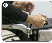
On '91-'05 Install shock studs, use nut from original shock studs. 06' and UP use your shock stud. Use blue loctite.
