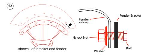
14.Remove top two star plate to spoke bolts and two bolts just below bolts previously removed, on one side at a time. Install fender and bracket on the rear end. Apply blue loctite. Install top two star plate bolts. Install lower mounting bolts on fender bracket. Install fender and fender bracket on other side as previously described. Torque upper fender bracket bolts to 60 ft. lbs. Torque lower fender bracket bolts to 60 ft. lbs.
