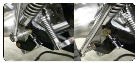
18. Hook up stock brake line, bled rear brake, tighten lug nuts on rear wheels torque 78 to 85 ft. lbs. and go for a ride. Re-torque lug nuts after 25 miles or 100 mile maximum.
