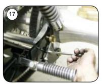
17. Torque the four rear end mounting bolts to 60 ft. lbs.
